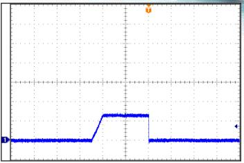
Figure 14: Output Short Load Current (50A/div) as a function of time (20ms/div) when the converter attempts to turn on into a 1 m $\Omega$  short circuit.
