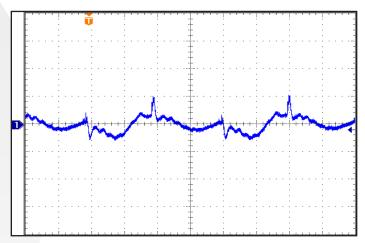
Figure 10: Output Voltage Ripple, Vout, at nominal input voltage and rated load current (50 mV/div). Load capacitance: 1μF ceramic capacitor and 100μF electrolytic capacitor. Bandwidth: 20 MHz. See Figure 13.
