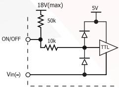
Figure B: Internal ON/OFF Pin Circuitry
