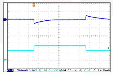
Figure 11: Output Voltage Response to Step-Change in Load Current (50%-75%-50% of lout(max);  $dI/dt=0.1~A/\mu s$ ). Load cap:  $1~\mu F$  ceramic and  $100~\mu F$  electrolytic capacitors. Ch 1: Vout (500mV/div), Ch 2: lout (20A/div).
