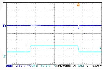
Figure 12: Output Voltage Response to Step-Change in Input Voltage (250V/ms). Load cap: 330  $\mu$ F electrolytic output capacitance. Ch 1: Vout (2V/div), Ch 2: Vin (50V/div).
