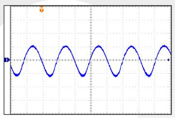
Figure 9: Input Terminal Current Ripple, i<sub>c</sub>, at full rated output current and nominal input voltage with SynQor MCOTS filter module (2 A/div). Bandwidth: 20MHz. See Figure 13.
