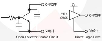
Figure A: Various Circuits for Driving the ON/OFF Pin
